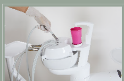
● 手机插入消毒配件专用位置 Insert the handpiece into the special position for disinfection accessories
